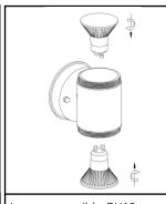
Insert compatible GU10 lamps by twisting securely into place.
