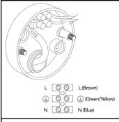
Connect supply to connector block, use additional connector block if loop permanent required.
