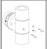
Reattach lamp covers and bolts, ensuring cables within enclosure and not trapped
