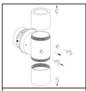
Unscrew bolts and lamp covers, ensure components are undamaged
