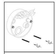
Using suitable fixings, screw the base to surface, threading cable(s) through hole in process
