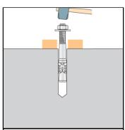
Insert expansion bolt into hole, with nut and washer attached.
