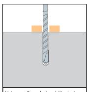
Using an 8mm hole, drill a hole 50mm deep for best results (where possible)
