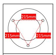
Mark 3 holes, 215mm apart in the shape of a triangle
