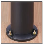
Remove nuts and washers from bolts. Place bollard over three bolts, ensure it is level
