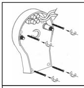
Using suitable fixings, screw the base to surface, threading cable(s) through hole in process
