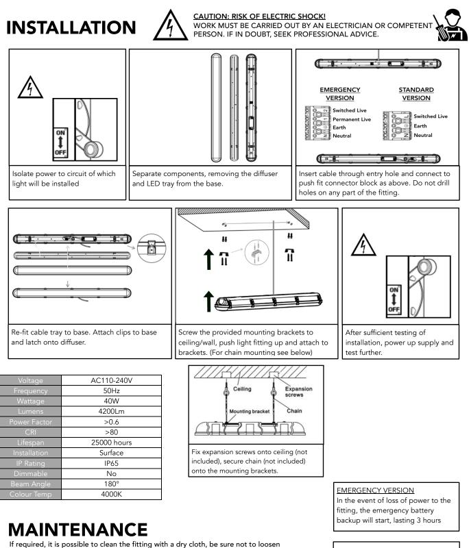
If required, it is possible to clean the fitting with a dry cloth, be sure not to loosen any components whilst cleaning. If essential to remove diffuser to clean, isolate power first.
