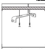
Loosen screws, twist and lift to remove mounting bracket from base
